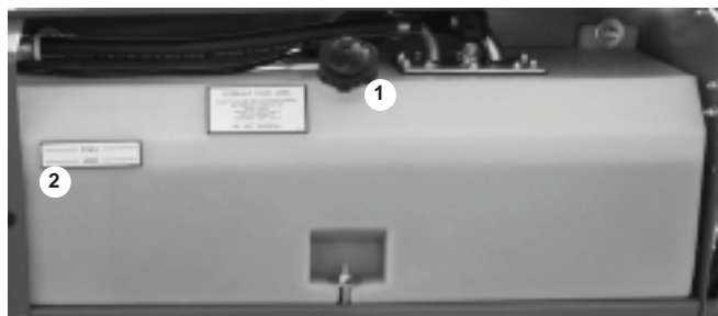
Figure 7.13 - Hydraulic Oil tank
