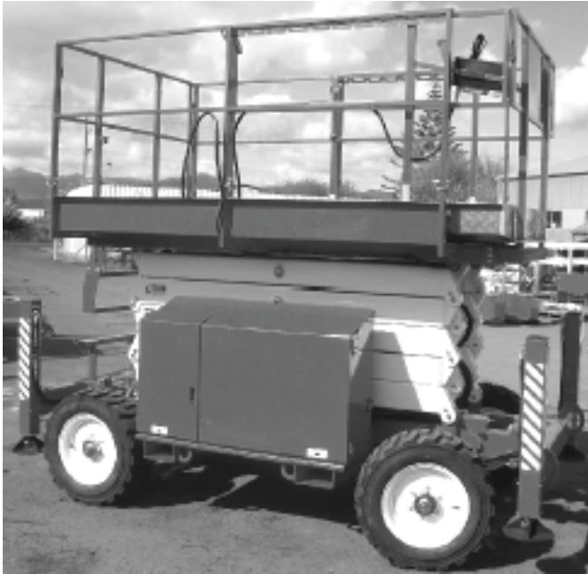
Figure 10.1 - Correct Stowed Position
