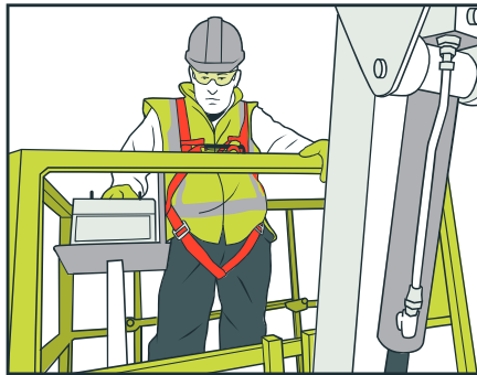
Figure 11: Inspect the MEWP before use
