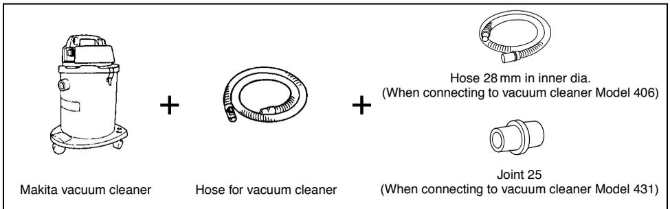
When connecting to Makita dust collector (Model 420), the optional hose or joint is not necessary. You can connect the belt sander directly to the hose of the dust collector.
