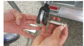
SECURING / REMOVING THE HYDRAULIC CYLINDER TO STOWAGE BRACKET WITH CLEVIS PIN FIG E
