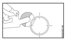
Second lateral cut in the marked area – never cut into the area of the last cut, to ensure a firm hold on the part of pipe to be cut
