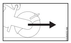
The cut-off machine pulls forwards, away from the user, when the abrasive wheel touches the object to be cut from above.
