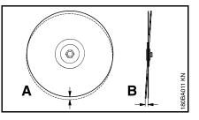
An excessively high radial run-out deviation (**A**) overloads individual diamond segments, which overheat in the process. This can lead to stress cracks in the parent wheel or to annealing of individual segments.
