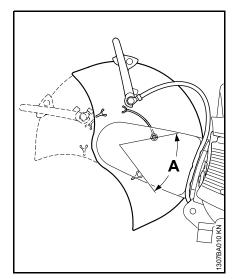
Rotate the guard forwards and backwards as far as possible – adjustment range (A) must be limited by the stop pin
