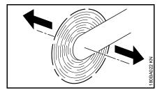
When a cut-off machine with an abrasive wheel rotating is moved in the direction of the arrow, a force is produced which causes the machine to tip sideways.
