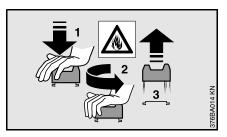
Never use a tool to open or close the bayonet filler cap. The cap can be damaged and fuel may escape.
