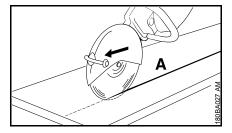
Work along the cutting line. When making corrections, do not tilt the abrasive wheel, but always set the abrasive wheel against the workpiece anew – the cutting depth for each operation should not exceed 5 to 6 cm. Cut thicker material in multiple operations
