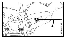
to tighten the ribbed V-belt, fit the combination wrench over the tensioning nut as illustrated
