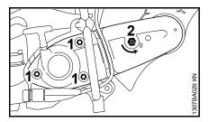
Prior to tensioning of the ribbed V-belt, the nuts (1) must be loosened and the arrow on the tensioning nut (2) must point to  $\mathbf{0}$ .
