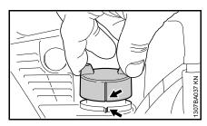
Grip the cap – the cap is closed properly if it cannot be removed and the markings (arrows) on the cap and fuel tank are aligned If the cap can be removed or the markings do not align, close the cap again – see sections "Closing the filler cap" and "Checking the lock".
