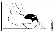
Set the abrasive wheel guard correctly: Guide particles of material away from the user and machine.
