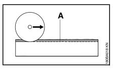
Grind a guide groove (A) along the line marked
