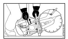
Place the cut-off machine carefully on the ground, ensuring that the abrasive wheel cannot touch the ground or any objects. There must not be anyone within the swivel range of the cut-off machine
