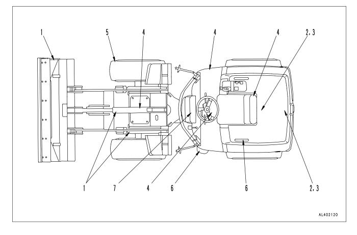
1. Check for damage, wear, play in work equipment, cylinders, linkage, hoses
