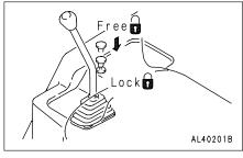
7. Lock work equipment control lever (6) with safety lock (7).
