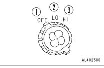
7. HEATER SWITCH Position ①: OFF Position ②: Lo Position ③: Hi
