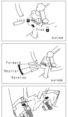
6. Release brake pedal (4), then depress accelerator pedal (8) to move the machine off.
