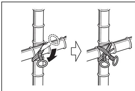
**NOTICE:** When you make the second tie, bend the tail of the first tie before making the second tie. Otherwise, the wire may be repelled a second time. It may cling to the tool tip, and the hook may be damaged.
