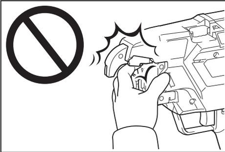
When you press the power button, the power turns on and the tying mode lamp lights up. In order for the tool to adjust its initial position, it operates temporarily. When adjustment has completed, the tool stops automatically. When you press the power button again, the power turns off and the tying mode lamp goes out.
