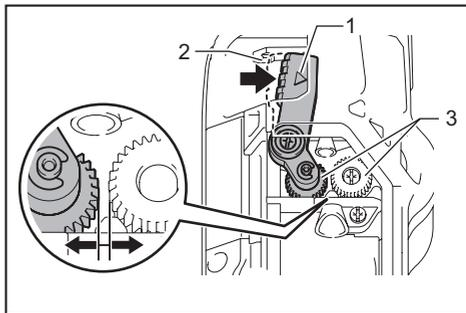
► 1. Release lever 2. Lock lever 3. Feed gears
