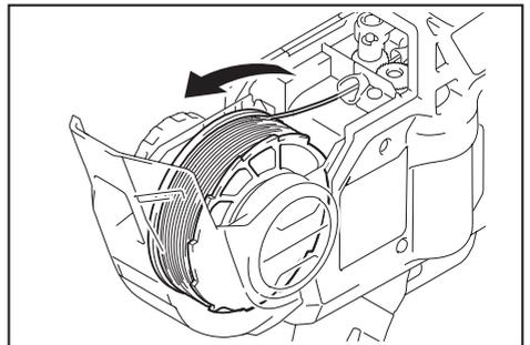
8. Release the lock lever. The release lever returns, and the wire is held by the left and right gears.
