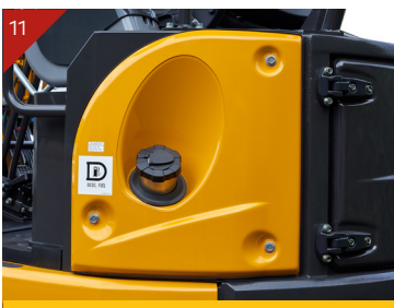
Fuel refill located in a convenient position
